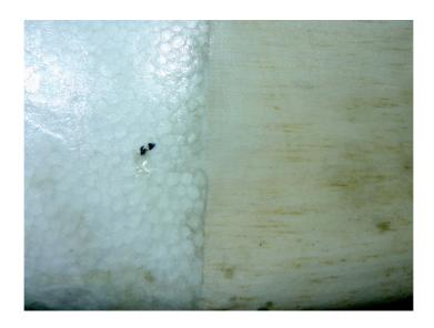
One word of warning. Eze-Kote does not stick to foam as well as to wood. It only matters if you want to put patterns in the finish. A single colour is fine. However masking tape might well pull the coating off the foam when you remove it. It would probably be best to use a plastic film instead of masked painting.
