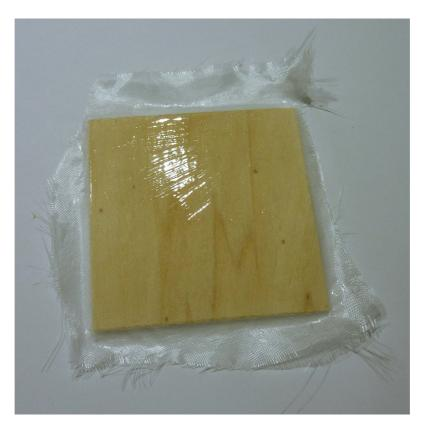
The surplus at the edges can be sanded off or cut with a very sharp blade and the whole piece given a final sanding to flatten it for painting. I used acrylic but the makers say it will take any paint.
